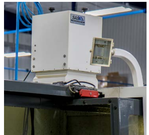
Mist Collector installed directly on CNC machine (Model 300 pictured).
