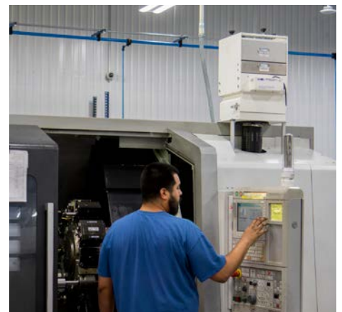
Mist Collector installed directly on CNC machine (Model 300 pictured).
