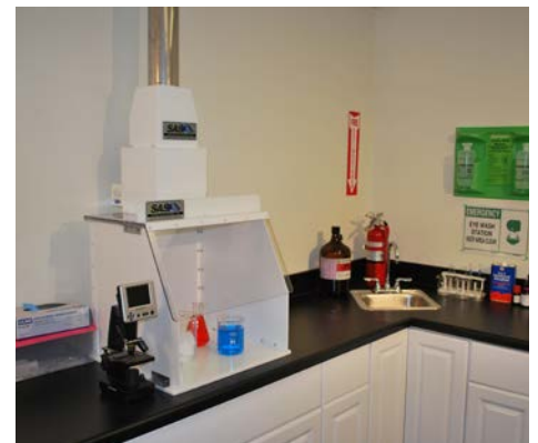
Mounted Sentry with Plenum can be used to exhaust out harmful fumes and particulate.
