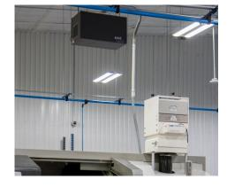
Model 2000 Ambient Mist Collector provides additional support for mist collection in CNC machine shops.
