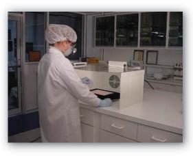
**The Winged Sentry** is a unique powder extraction unit that features infinitely adjustable side flaps for optimum source capture.
