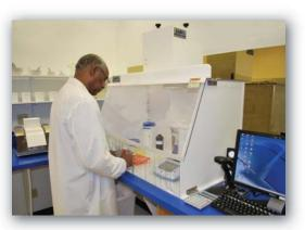
**Pharmaceutical Containment Hoods** come in a variety of sizes and are equipped with powerful fans and high-quality HEPA filtration media.
