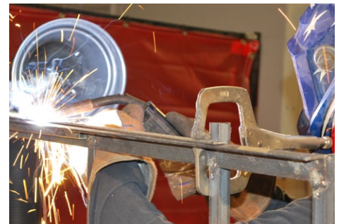
The self-supportive flex arm on the Model 300 Welding Fume Extractor allows the operator to easily adjust to capture fumes at the source.
