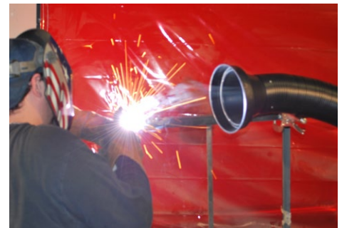
The self-supportive flex arm on the Model 300 Welding Fume Extractor allows the operator to easily adjust to capture fumes at the source.
