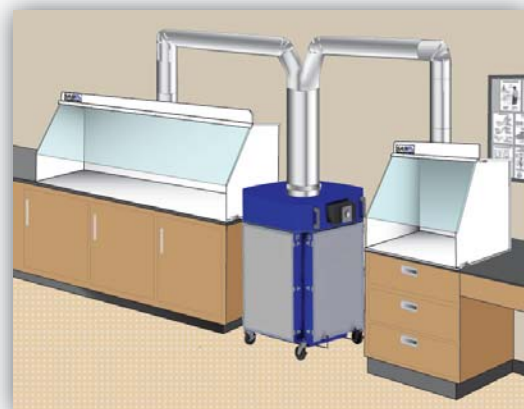
Conceptual Drawing - Chemical Fume Removal in a Laboratory Environment with Sentry Air Systems Exhaust Hoods
