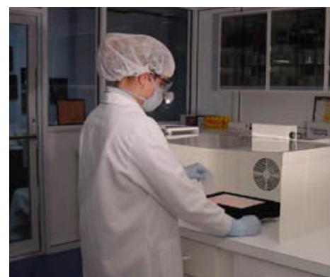
The Model 300 Winged Sentry with lid extracts fumes and particulate for a variety of laboratory and medical applications.
