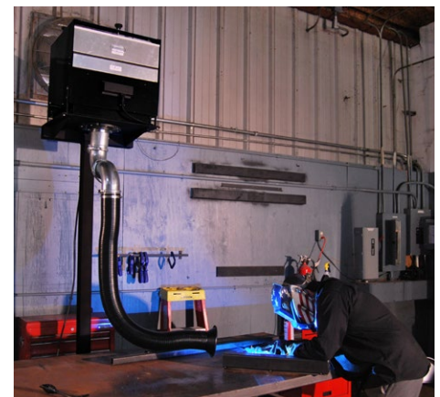
Model 450 Mounted Sentry frees up valuable benchtop space with fume extractor stand.
