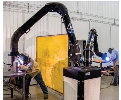
This powerful fume extractor can help protect two operators from chemical fumes, shown here being used for welding.
