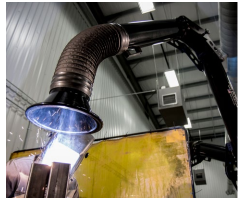
This powerful fume extractor can help protect two operators from chemical fumes, shown here being used for welding.
