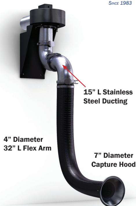
Fan-Powered Flexible Fume Extraction Arm
