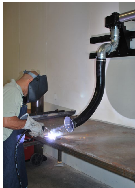
The Fan-Powered Flexible Fume Extraction Arm source captures fumes and can connect to existing ductwork.
