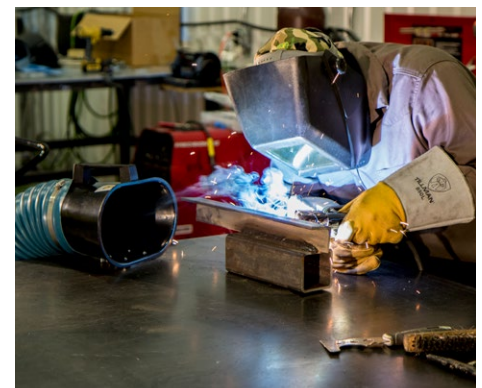
The magnetic capture hood can attach to surfaces to allow hands-free source capture fume extraction.
