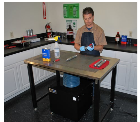
The Industrial Downdraft Bench provides fume extraction for use with chemicals, solvents, and aerosol sprays.
