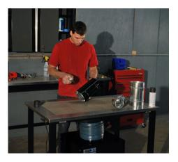
The Industrial Downdraft Bench provides fume extraction for use with chemicals, solvents, and aerosol sprays.
