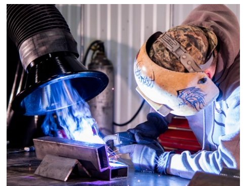
The Heavy Duty Arm allows the operator to move it closer to the fume source.
