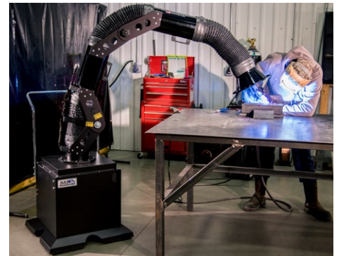
The Heavy Duty Arm allows the operator to move it closer to the fume source.
