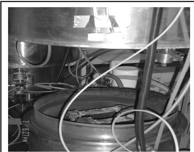
FIGURE 2. Reactor cleanout process with no fume extractor (LEV)
