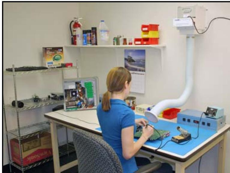
^The **Sky Sentry [SS-200-SKY]** is designed to hang over the workspace area to capture particulate. The semi self-supportive flex allows the operator to place the source capture area where it is needed the most.
