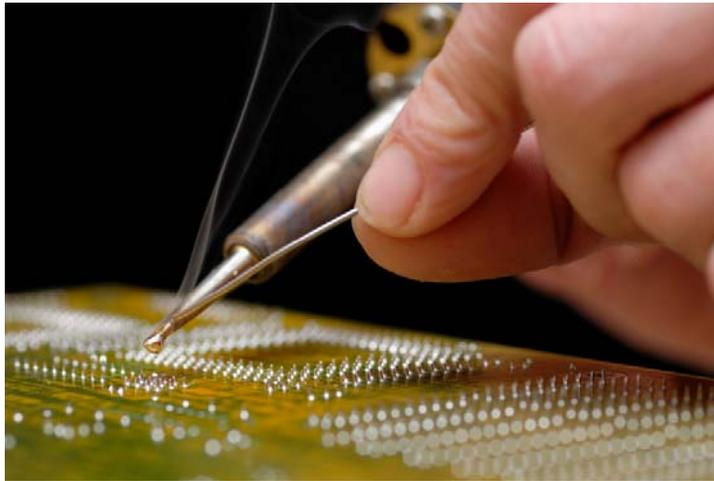
Soldering is the process of combining two metals via a third metal (the "joint") with a lower melting point than the base metals. In this procedure, the two base metals are not distorted and only the filler metal is melted. There are numerous filler metals, or solder, available for soldering applications. For the purpose of narrowing the content of this report, only lead-based solder and rosin-based flux will be discussed.
