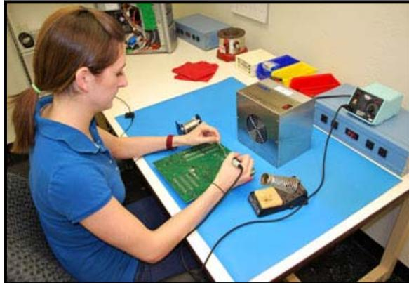
^The **Stainless Steel Solder Sentry [Model SS-100-SS-ST]** is perfect for desk-top soldering. This ESD-safe unit is equipped with a powerful fan and filtration system that captures contaminants and redistributes them as purified air.
