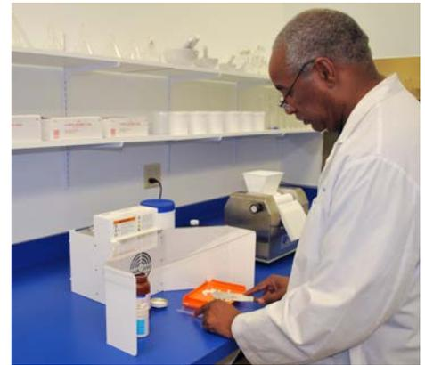
The Model 200/225 Winged Sentry with lid extracts most of the airborne particulate for pharmaceutical applications.
