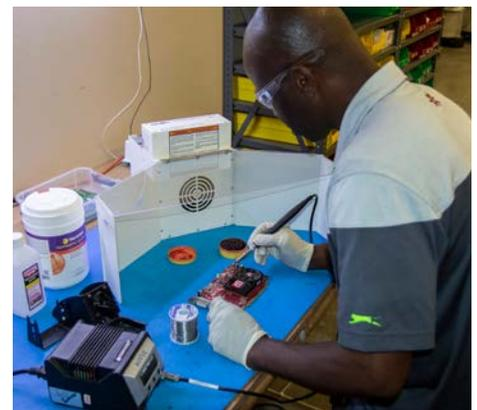
The Winged Sentry with lid helps protect the operator from harmful soldering fumes.
