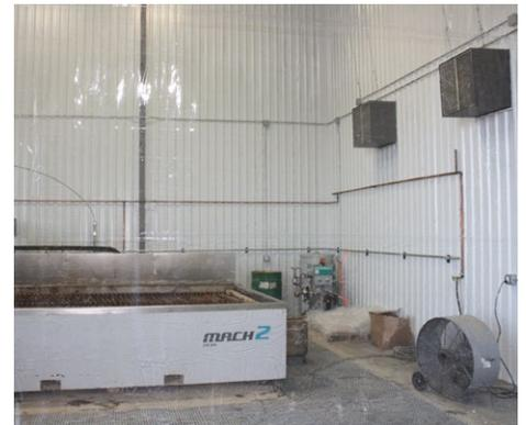
*Model 2000 Ambient Mist Collector collects more than just oil mist, this system can be used for waterjet machines.*
