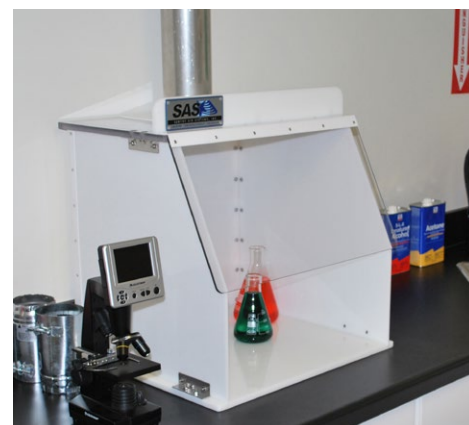
Ducted Fume Hoods provide fume extraction for lab and chemical use.
