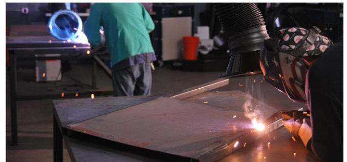
The powerful fan and cleanable filter media in the Model 500/550 Dual Stand Assembly can help protect two workers from welding fumes for heavy-loading applications.
