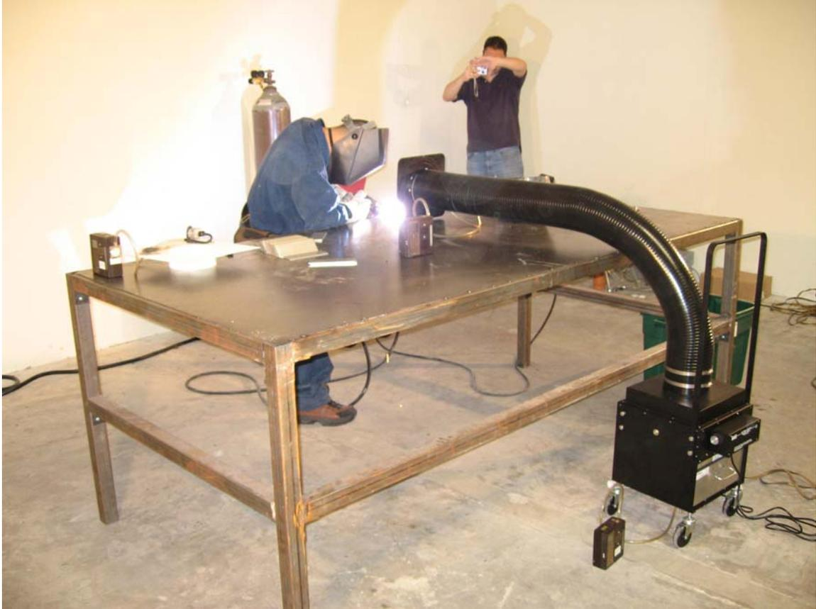
**Photograph #4: The Sentry Air Systems Model 300 welding fume extractor is shown in operation above while the welder is welding 316 stainless steel. Air sampling pumps can be seen on the work table as well as at the inlet and outlet of the fume extractor. The Welder is also wearing a pump and sampling cassette to measure Cr<sup>+6</sup> in his breathing zone.**
