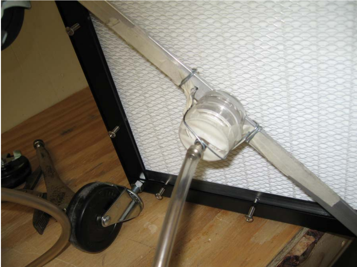
Photograph #2: The sampling filter cassette is shown above, mounted on a support brace to hold the cassette in the exhaust stream from the welding fume extractor. A hole was drilled in the brace to allow the cassette to sample the exhaust air stream.
