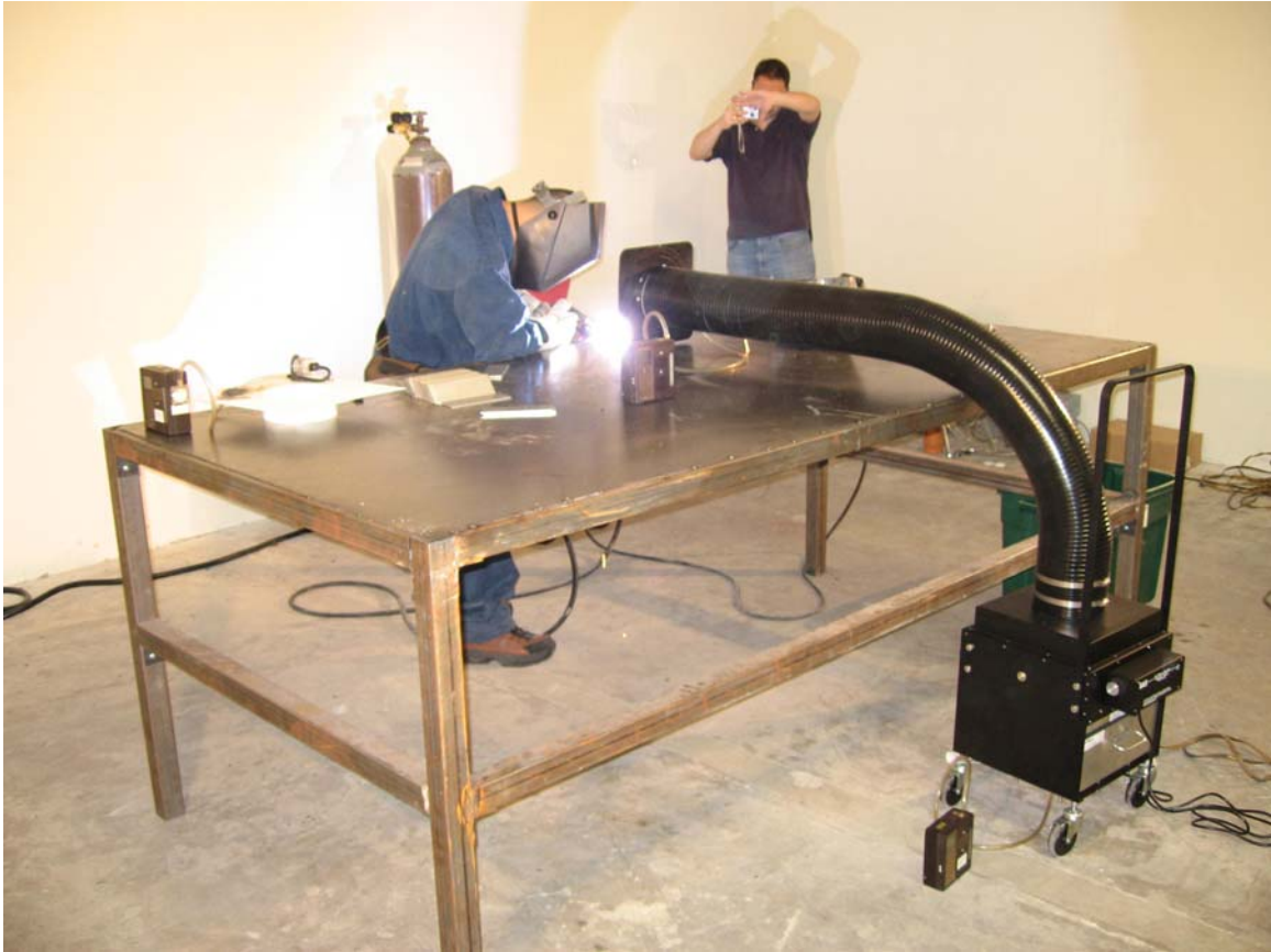
Photograph #4: The Sentry Air Systems Model 300 welding fume extractor is shown in operation above while the welder is welding 316 stainless steel. Air sampling pumps can be seen on the work table as well as at the inlet and outlet of the fume extractor. The Welder is also wearing a pump and sampling cassette to measure Cr +6 in his breathing zone.
